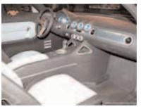
cabin. The belt line is comparatively high, so the seating sense is being surrounded by the vehicle. Interior accents combine leather and aluminum in a way that evoke an earlier time (say 1954) as well as the future (if not the present). Anticipating use to haul cargo, not only is there a sliding panel that moves over the tailgate, but the rear roof panel can be removed.
